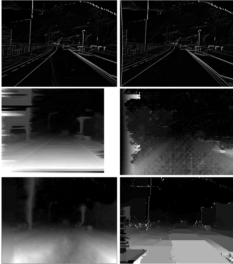
Fig. 4. Top: Sobel edge maps of the left-right stereo pair in Figure 1, used as stereo input pair. Middle: depth maps of single line DP (left) and Birchfield-Tomasi cost function in 8-ray DP (also known as SGM BT). Bottom: BP (left) and GC results.
