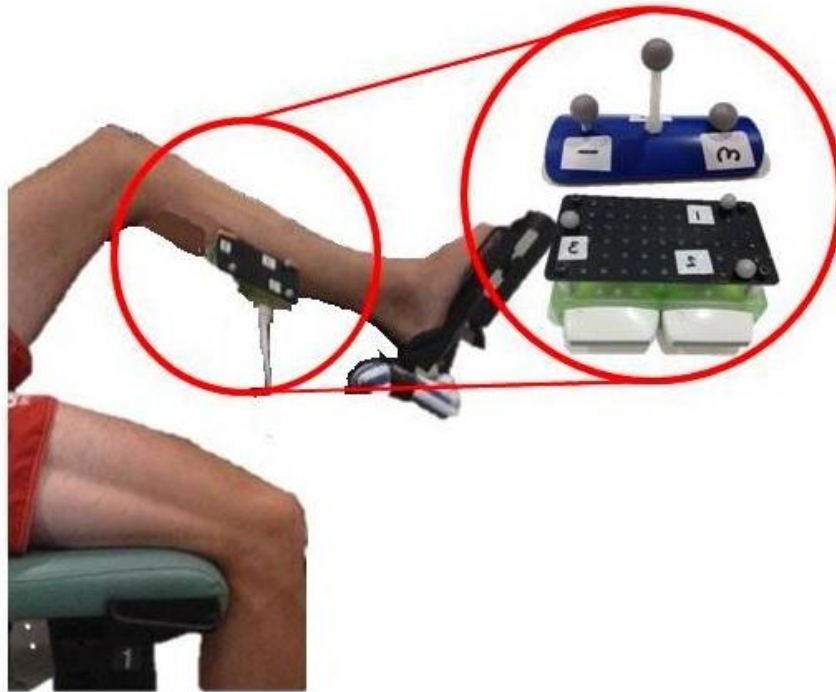
Figure 1: The experiment setup. Each subject was seated with the leg in a flexed pose and the foot was moved through dorsiflexion. Top right shows the triad of markers attached to the leg used to define the leg frame of reference. Markers are also attached to the ultrasound transducer to define the imaging plane.
