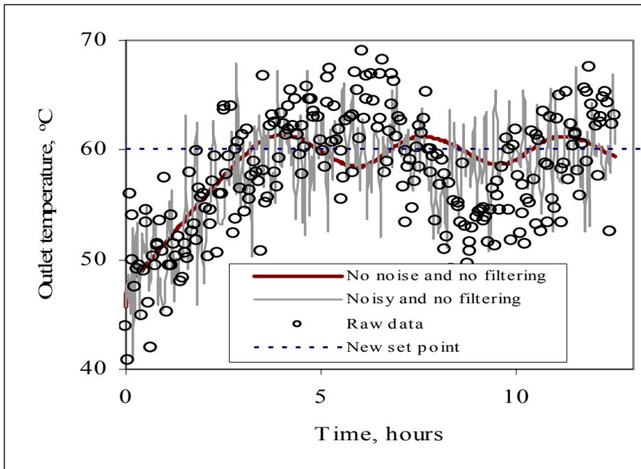
**Figure 8. Outlet temperature response to a set point change, PID controller with data reconciliation**
