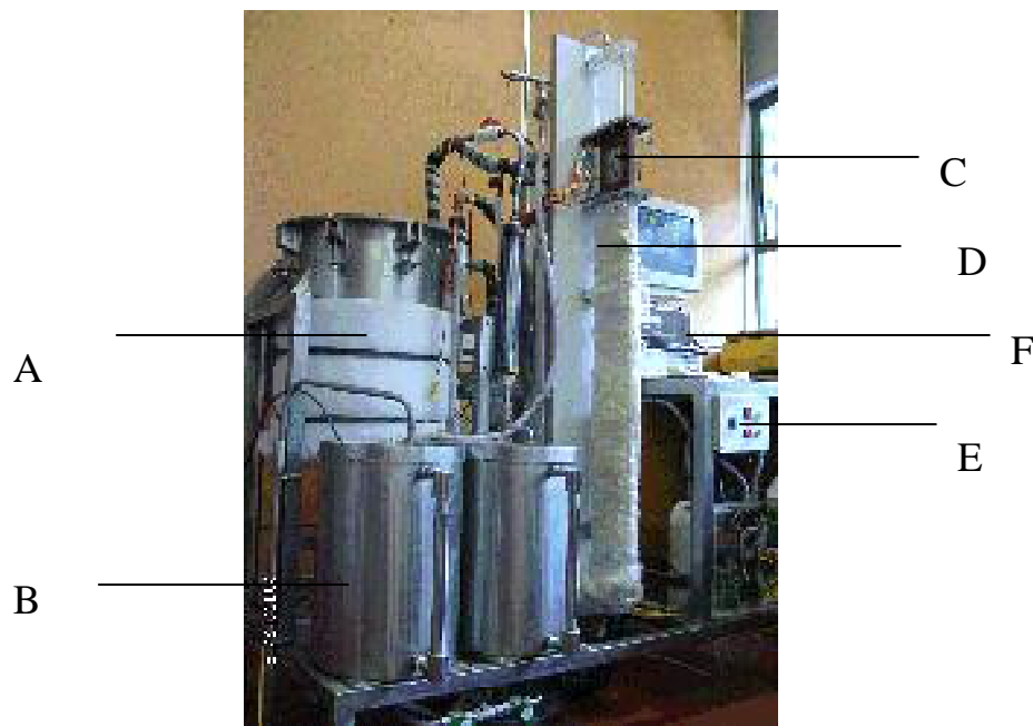
Figure 1: The photo of fouling apparatus: milk tank (A), cleaning solution tank (B), fouling test section (C), reference section (D), control equipment (E) and data recording equipment (F).
