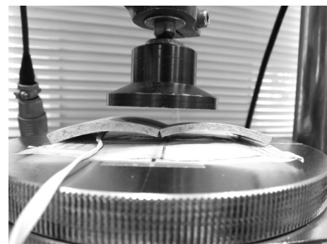
Fig. 10 Condition of A1-segment (thickness of segment: 5 mm) after loading in simple bending test.
