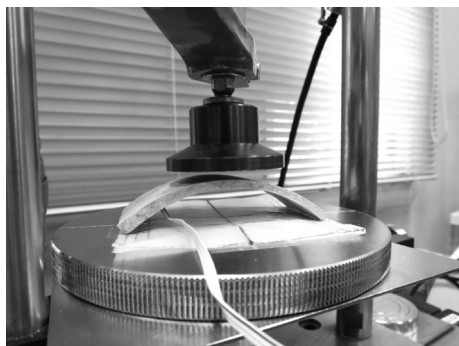
Fig. 4. Condition of A1-segment (thickness of segment: 5 mm) in simple bending test before loading.
