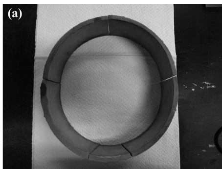
Fig. 3. Small-scale physical model of the segments (thickness of 5 mm). (a) Segmental ring, (b) K-segment (The angle of the sides of K-segment adjacent to the B-segments was 9.7 degrees).
