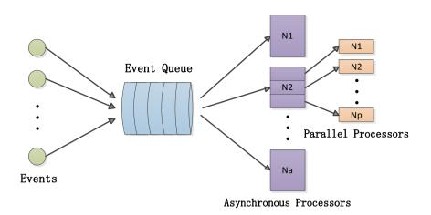
FIGURE 1 A parallel event dispatching model that has multiple asynchronous processors and parallel processors.
