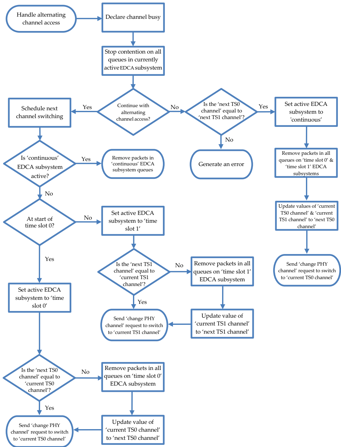
Figure 4.29: The MAC layer handling alternating channel access
