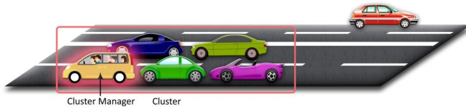
Figure 2.2: A vehicle forming a cluster to select a common control channel
