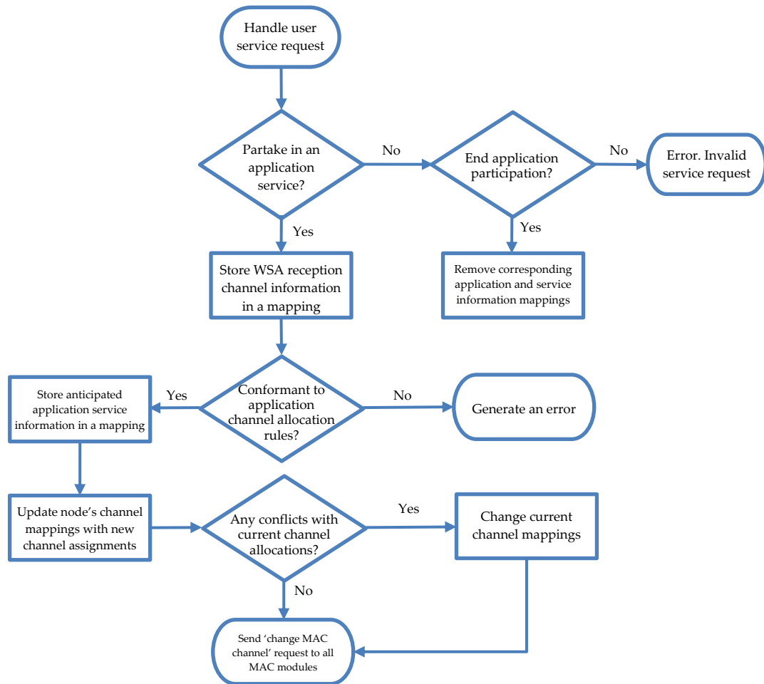
Figure 4.19: The process of handling a user service request
