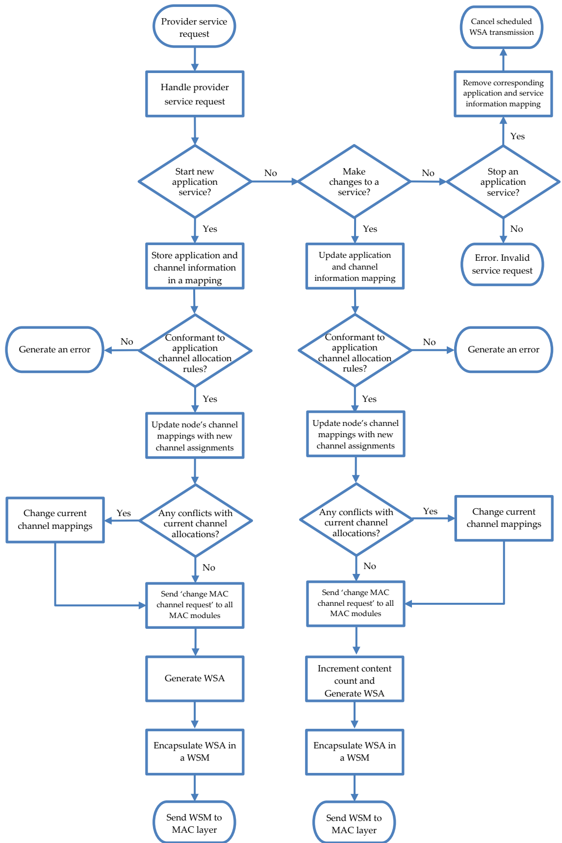
Figure 4.17: The service provider role of WAVE 1609.3 module
