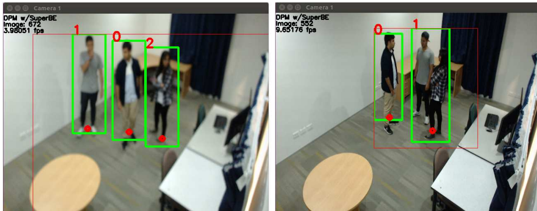
Figure 5.11: Two examples of difficult frames; on the left, the camera has gone out of focus, blurring the texture descriptors, while on the right, the person detection algorithm has drawn a single bounding box that actually contains two people, introducing erroneous/noisy data into the classification and model update process.
