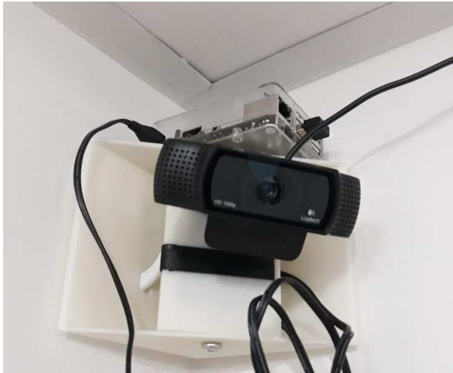
Figure 7.2: A photo of the prototype smart camera used in the video analytics system. The cables leading out of the figure only provide power.
