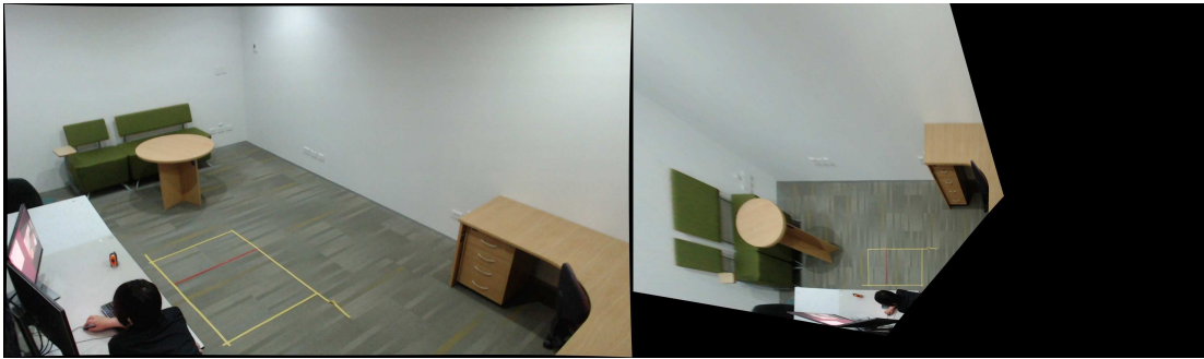
Figure 5.2: An example of the effects of camera calibration on camera view 1 from UoA-Indoor, with the transformation matrices from intrinsic (left) and extrinsic (right) calibration applied.
