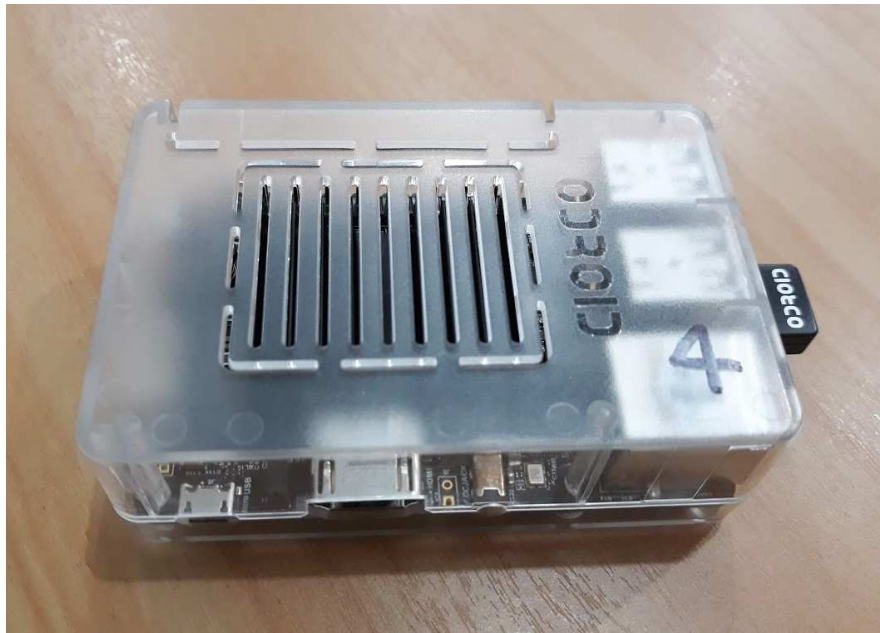
Figure 7.1: The ODROID-C2 board in a plastic case with a USB Wi-Fi adapter.
