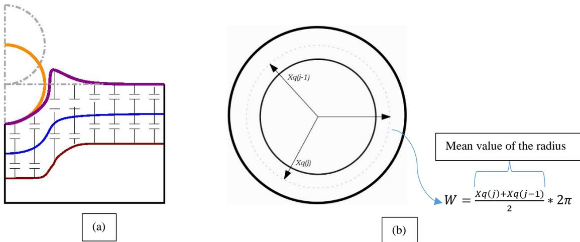
Figure 2. (a) The overview of the indenter and the proposed DE sensor deformation with the capacitance layout due to load applied. (b) The top view of the indented sensor area.
