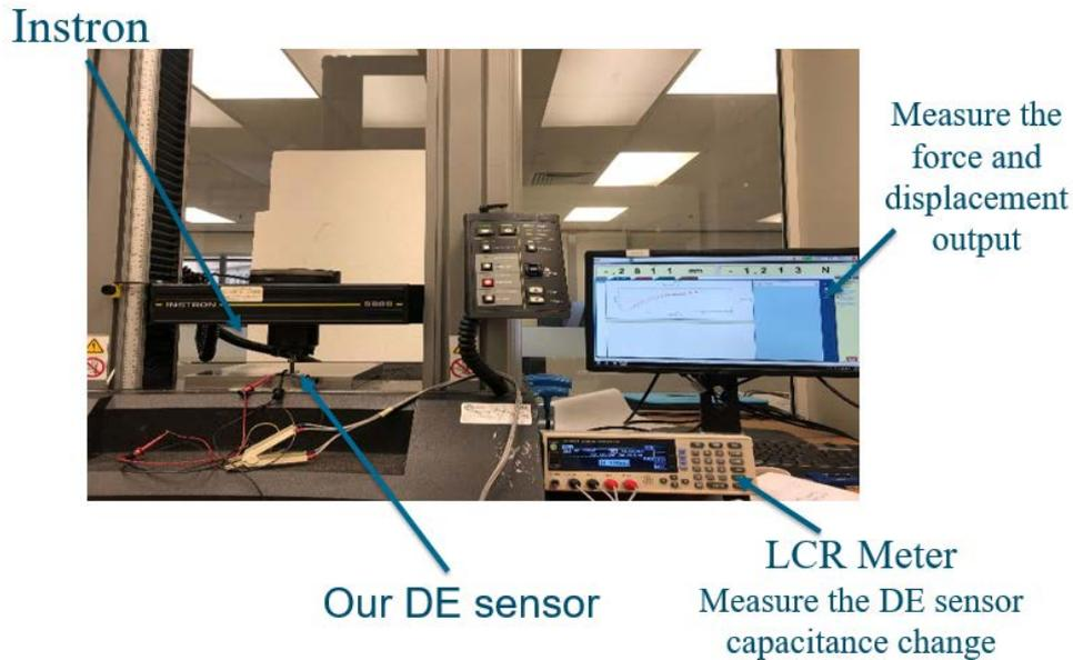
Figure 3. Measurement setup: Instron machine-applied different forces with an indenter in the designed sensor to record displacement and LCR Meter to monitor the sensor's capacitance change.
