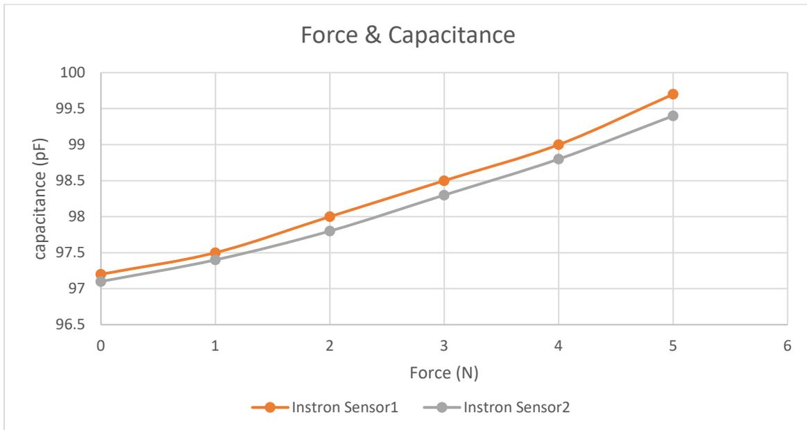
Figure 5. Change in sensor capacitance as a function of applied force on the indenter. (by Instron & LCR Meter)
