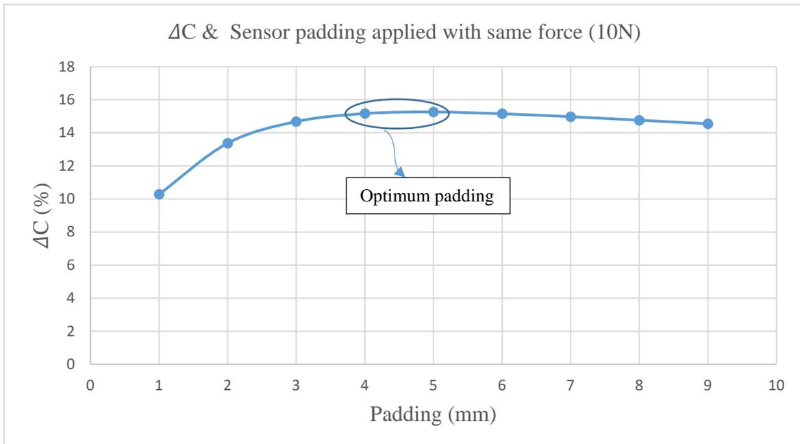
Figure 7. The modelling results of the Delta C changes when 10N load applied in the padding with different thickness
