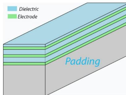
Figure 1. Overview of the shielded capacitive DE sensor with padding
