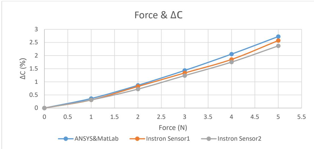
Figure 6. The Delta C changes between the ANSYS modelling results and the experimental test results (by Instron & LCR Meter)
