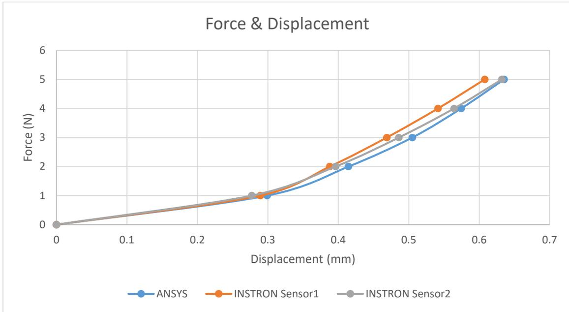
Figure 4. Comparison of FEM simulations with experimental compression measurement using an Instron universal tester. The total thickness of this sensor is 1.84mm, which includes the sensor padding of 1.1mm
