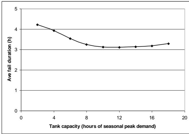
**Figure 3** Average tank failure duration as a function of the tank capacity
