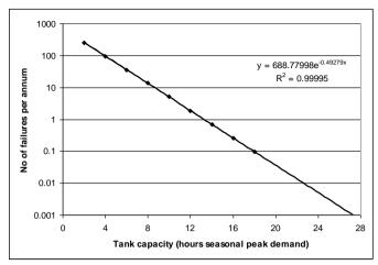
Figure 2 Annual average number of tank failures as a function of the tank capacity
