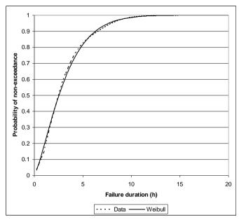
**Figure 4** Failure duration distribution for a tank with a capacity of 12 h of seasonal peak demand.
