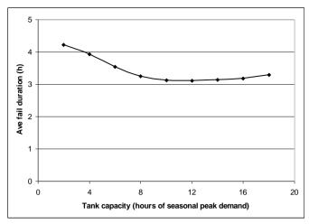
**Figure 3** Average tank failure duration as a function of the tank capacity
