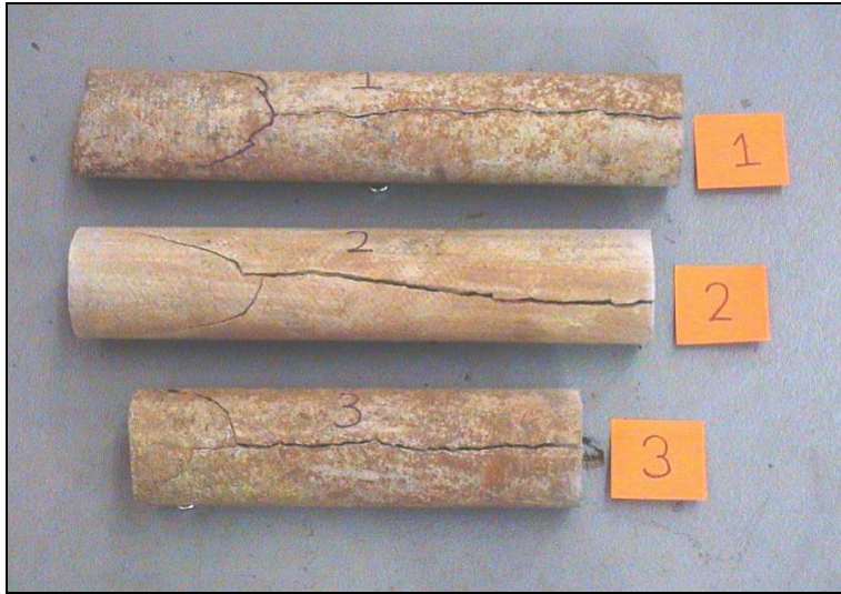
Figure 4 - Failed asbestos cement pipe sections
