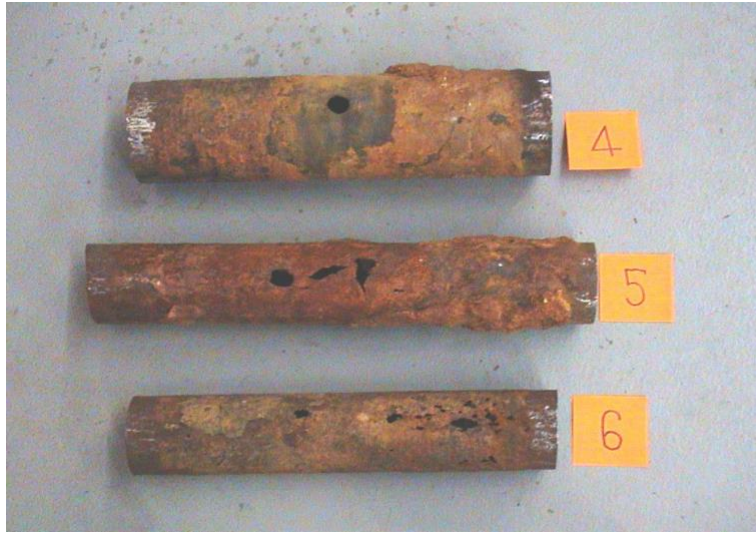
Figure 6 - Failed steel pipe sections
