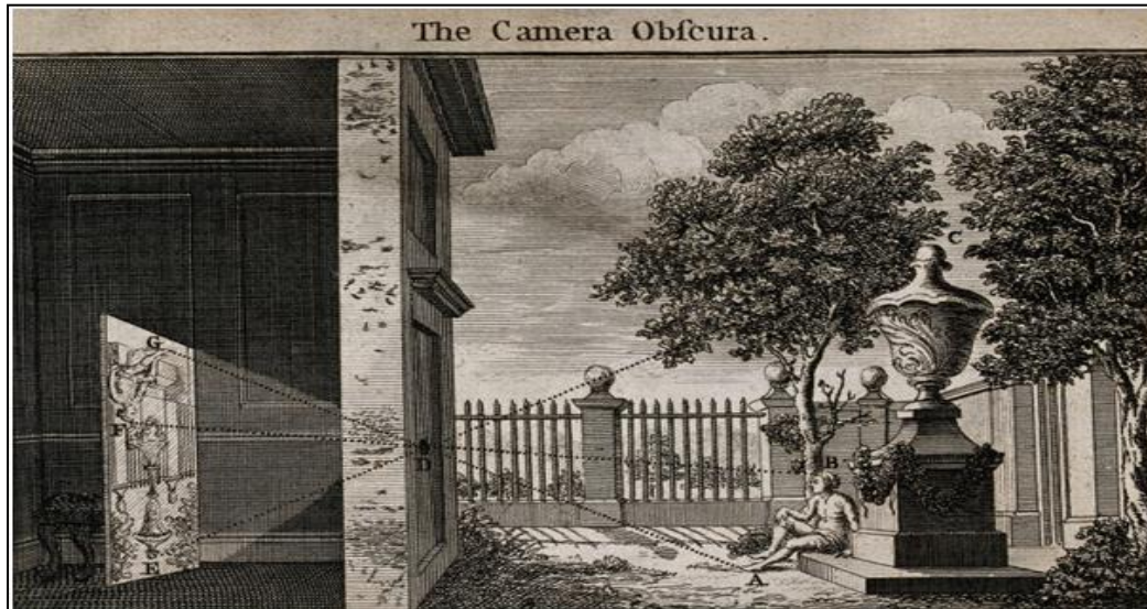
Figure 7. An engraving showing an operational camera obscura. "Optics: The Principle of the Camera Obscura," 1752
