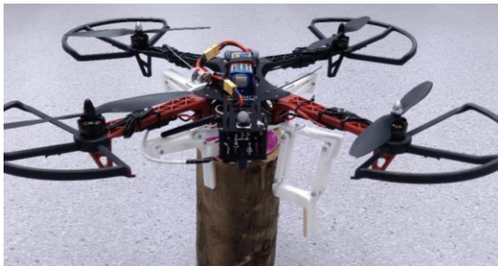
Fig 13: Partial engagement of passive mechanism on 150mm post
