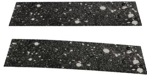
Fig. 3. 3D reconstructions of the speckled cantilever surface showing undeformed (0 N, top) and deformed state (9.81 N, bottom).
