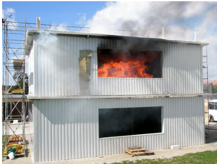
Figure 12. Experimental building during the Veselí Travelling Fire Test.
