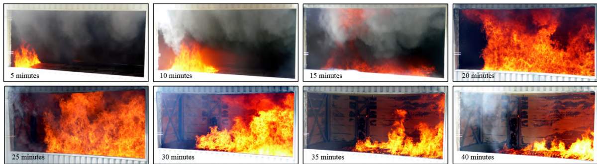
Figure 15. Fire development in the Veseli Travelling Fire Test 10 .
