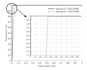
Figure 5. ROC curve and the corresponding AUC for the 11-layers WF-CNN gamma spike classifier
