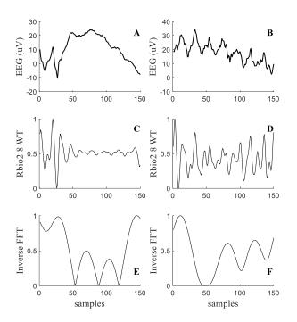
Figure 3. (A-B): Examples of non-spike ECoG background events. (C-D): The corresponding Rbio2.8 wavelet transforms of the ECoG segments in A and B at scale 7. (E-F): The corresponding inverse Fourier transforms of the ECoG segments in A and B using band-pass filter 80-120Hz.
