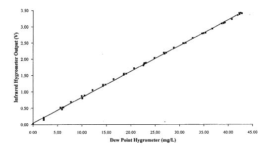
FIG. 4. Calibration with a dew-point hygrometer. Solid line is a linear fit to the data (r=0.9996).
