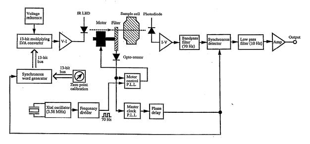
FIG. 2. Block diagram of the LED current driver electronics and the lock-in detection scheme.
