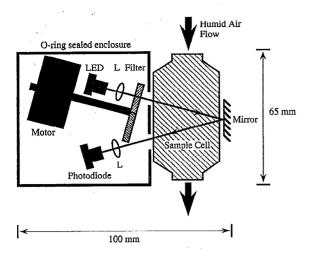
FIG. 1. Schematic of the optical layout.
