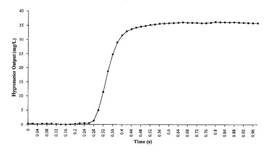
FIG. 5. Response time of the hygrometer.
