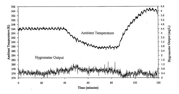
FIG. 7. Effect of ambient temperature on the hygrometer output.
