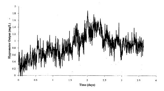
FIG. 6. Long-term stability, as measured with dry air.
