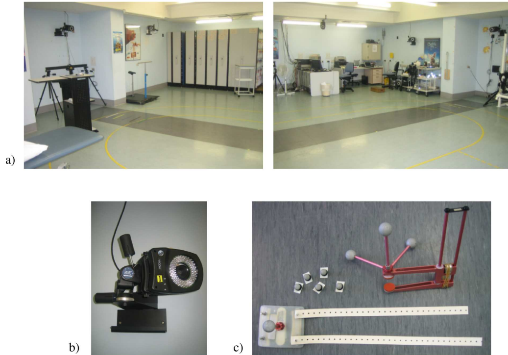
Figure 3.6: The Vicon MX motion analysis system at the Hugh Williamson Gait Laboratory, Victoria, Australia, showing a) the measurement field, b) an infrared camera and c) retro-reflective markers and different devices for attaching them.
