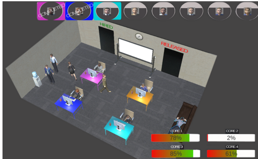
Figure 3: Screenshot of a visual analogy video (Video #2 from Table 1). It demonstrates the behavior of eight threads (workers) as they context switch on a system with four physical cores (desks), i.e., a quad-core processor. Each thread is assigned one of the coarse-grained tasks, shown at the top of the screen.
