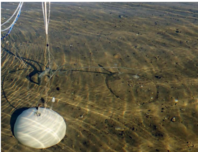
Figure 1.3B Small, in situ sediment incubation chambers. Half-sphere chambers are inserted 2 cm into the sediment once it is inundated to a tidal height of \sim 20 \text{ cm} , enclosing 0.025 \text{ m}^2 (17 cm diameter) of intact benthic habitat and 1.2 L of overlying water. Circular, lead weights sit about half way down the chamber to hold it in place (not pictured). Light chambers are clear while dark chambers are black with the outsides painted white to help keep the temperature uniform on sunny days. Approximately 2 m of sample tubing is attached to a port at the top of each chamber with a luer lock on the other end, allowing for sampling of the water within the chambers at the surface. One small port on the other side of the chamber lid ( \sim 3 \text{ mm} diameter) is left open so that sampling does not create negative pressure and pull out sediment pore waters. Light and dark bottles filled with ambient site water are also incubated (without bubbles) to account for any water column activity. Temperature and light loggers are staked to the sediment outside the chambers. While the surface area of these chambers is less than that of the large benthic chambers, it is larger than cores, thus likely capturing greater animal activity than core incubations.
