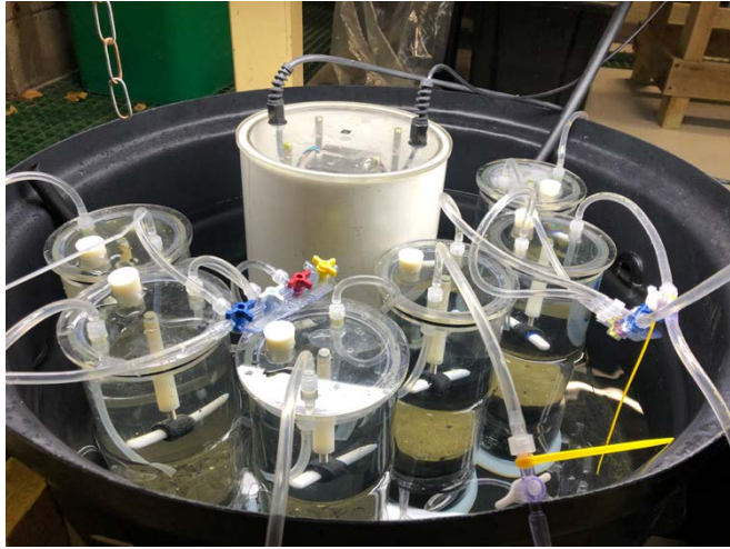
Figure 1.3C Intact core incubation chambers. Cores are inserted into the sediment in the field at low tide, removing a section of sediment with a surface area of 0.01 \text{ m}^2 , approximately 15 cm deep. Cores are then gently filled with 0.2 \text{ }\mu\text{m} filtered site water and placed in constant temperature, flow through water baths. Core lids are equipped with magnetic stirring bars, which are moved by a magnetic carousel in the middle of the water bath. The carousels turn at \sim 50 \text{ RPM} , slow enough to prevent sediment resuspension, but fast enough to prevent stratification. Inflow ports are attached to gas-tight bags of filtered site water on a table above, resulting in a gravity fed system that replaces any water that is removed for sampling without introducing any air, and creating sufficient head pressure to fill sample vials without suction. Silicone stoppers plug a hole in each lid which allows for removal of air bubbles in the capping process and for the deployment of various sensors if needed. Water baths can be kept open under lights to mimic light conditions, or covered with opaque sheeting for darkness. Temperature and light sensors are deployed at sediment height within each water bath. While cores capture the smallest surface area, they are ideal for performing more technical experiments where a controlled environment is needed.
