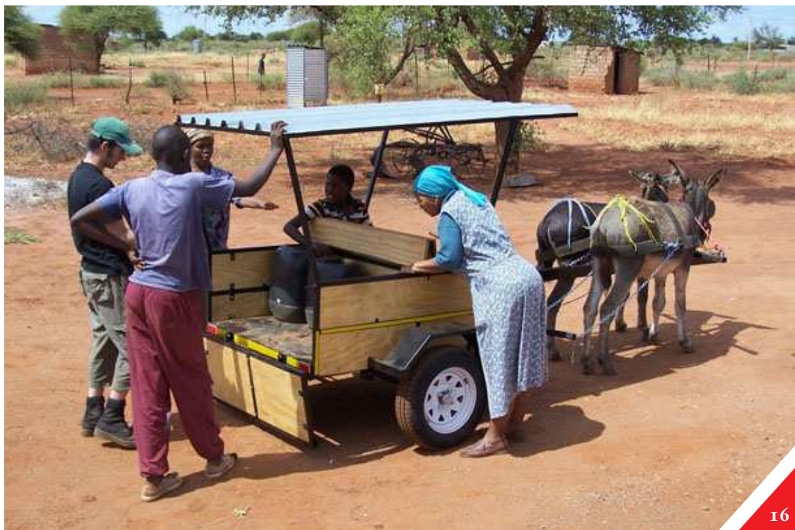
Figure 16: Community members testing the water carrying capabilities of the 'Tin Lizzy' single-axle donkey cart prototype, March 2007.
