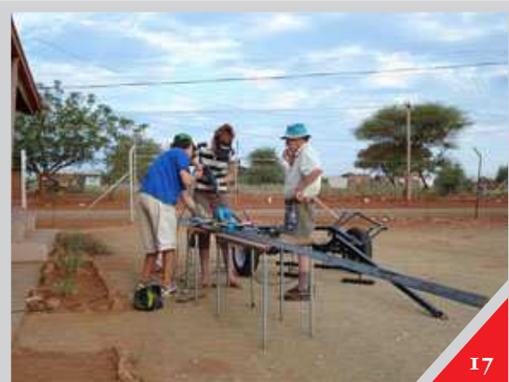
Figure 17: The dissel boom on the 'Plain Jane' donkey cart is shortened according to community feedback regarding its length, 2007.
