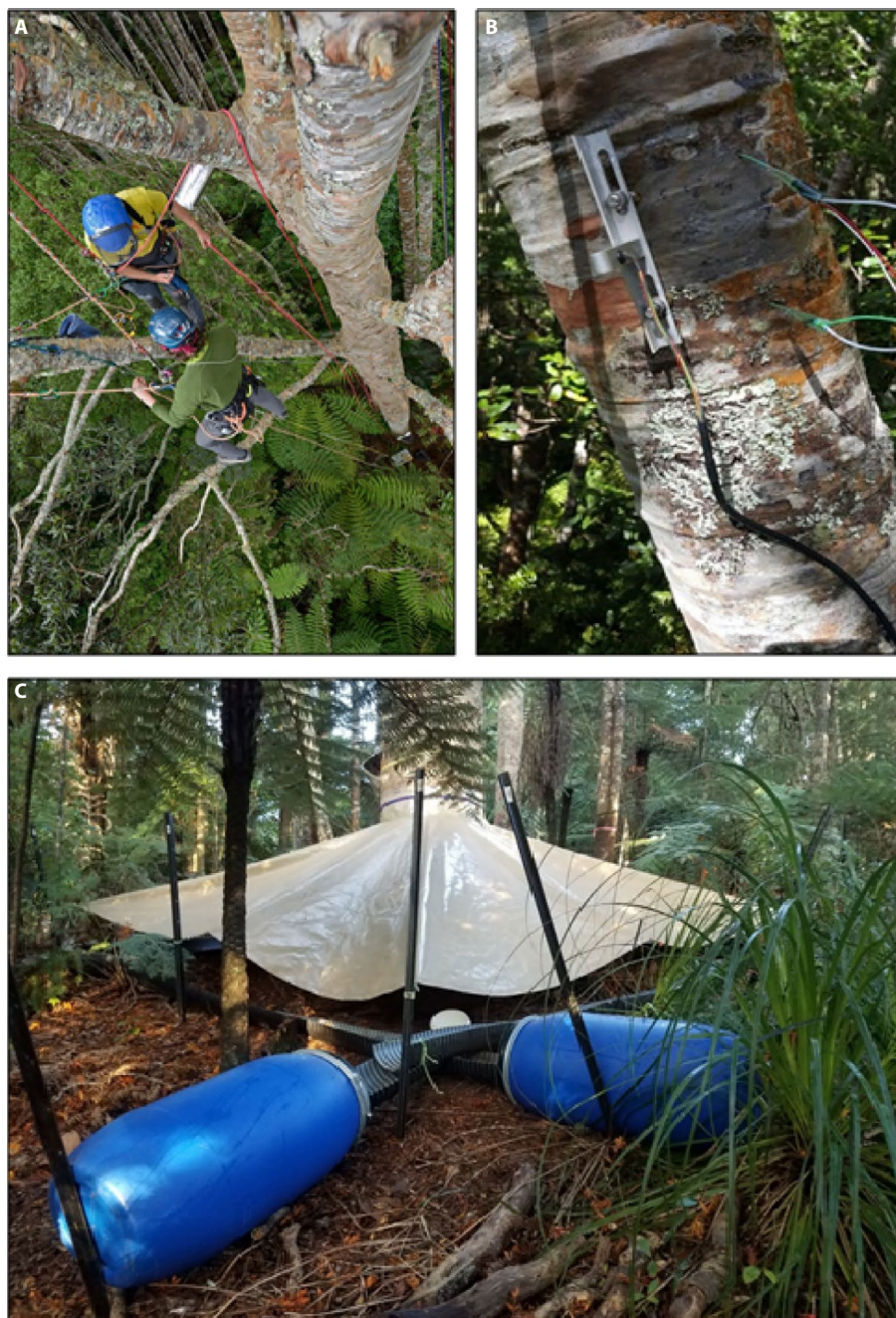
FIGURE 1. Canopy and base of tree installment stages of the drought experiment. Canopy access for installation of water relations instruments (A), point dendrometer (left) and sap flow sensor (right) installed in a branch (B), and the final set-up of a droughted tree showing the throughfall exclusion tarpaulin, culverts, and collection basins (C).
