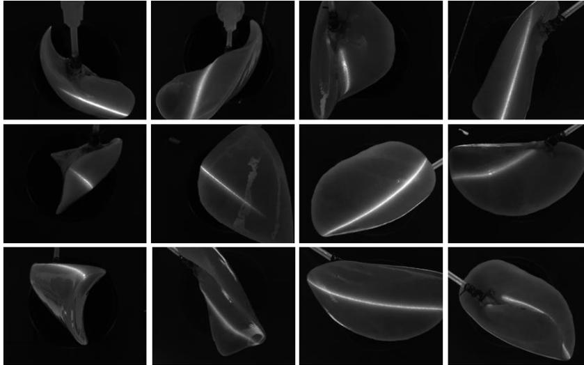
**Fig 4.** Examples of laser line images. The lungs were held at a fixed pressure while each line was acquired individually. In this data set, the lungs were held at 2000 Pa. Firstly, images of the lungs were taken at different levels of illuminations from LEDs, then 22 images were recorded of individual laser lines on the lungs.
