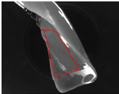
**Fig 8.** Region of interest for a reference camera selected on fresh lung. In the reference state the lung was inflated to 2069 Pa.
