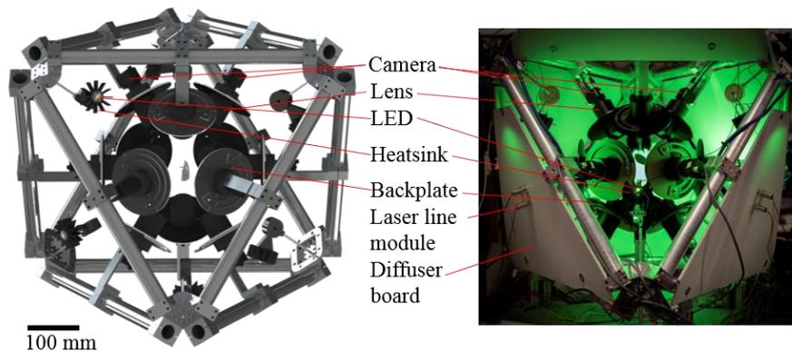
**Fig 3.** Frame constructed for performing full-field imaging of the lung surface during pressure-controlled inflation experiments. Left shows a CAD rendering of the stereo rig. Right shows the physical rig.
