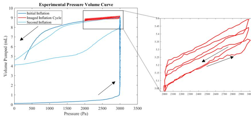
**Fig 2.** Left, PV loops from two full range inflations and an imaging cycle of three PV loops from 2000 Pa to 3000 Pa and back. Arrows depict the direction of increasing time. Right, expanded view of the three PV loops used for imaging.
