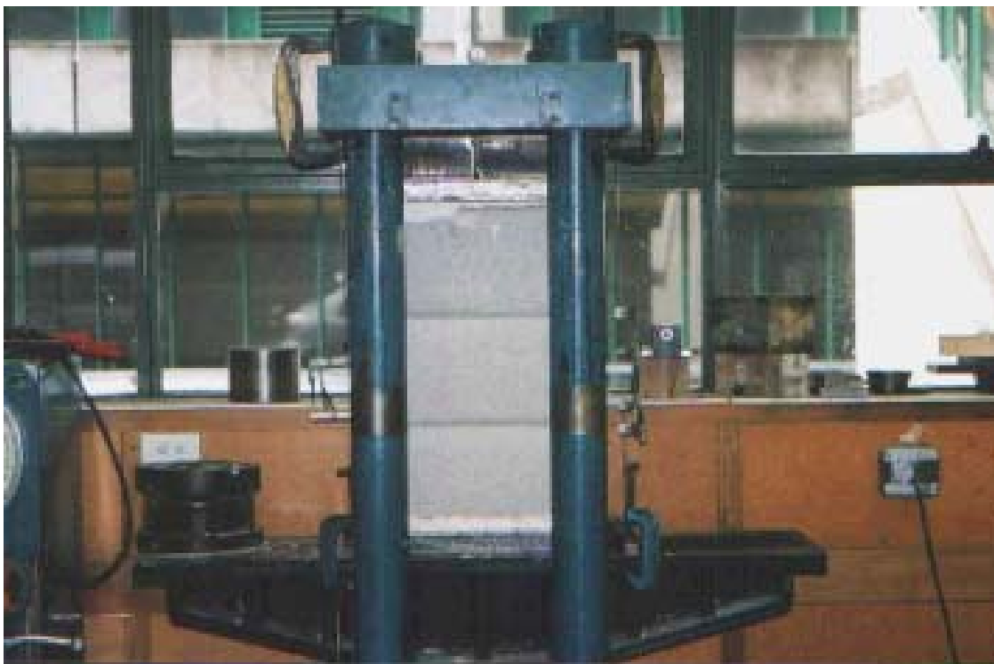
Figure 3.4 Masonry prism subjected to compression test.
