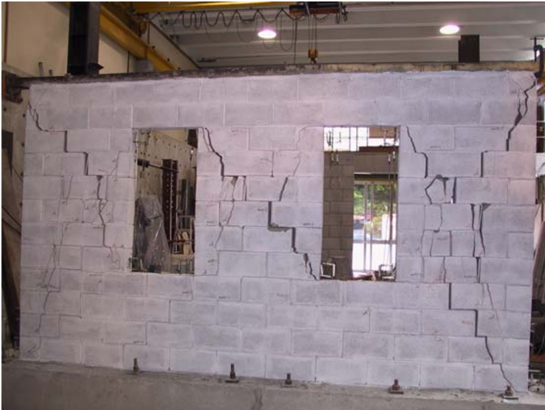
Figure 6.23 Series B, condition of Wall B6 at end of testing.
