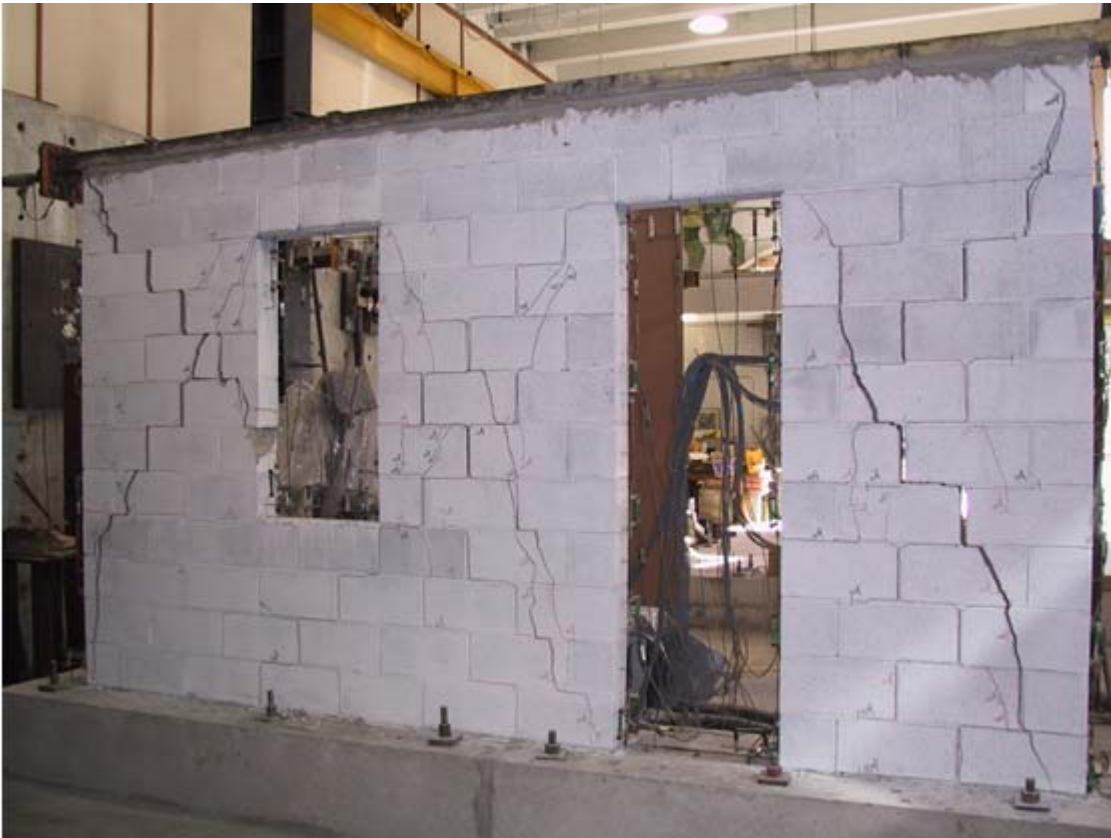
Figure 6.24 Series B, condition of Wall B8 at end of testing.
