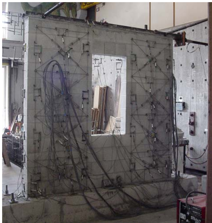
Figure 6.5 Instrumentation mounted on wall before testing.
