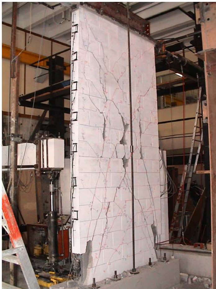
Figure 3.21 Series A, condition of Wall A9 at end of testing.
