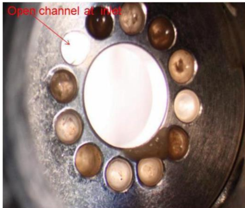
Figure 1.6 The inlet to the Water Processor Mostly Liquid Separator of the International Space Station, with biofilm formation at many of the channels. Image: NASA, (Zea et al., 2018).
