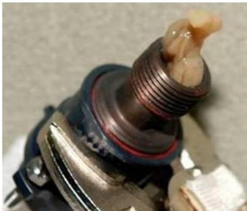
Figure 1.7 The inlet of the Russian condensate processor, with formation of biofilms inside the condensate plumbing. Image: NASA, (Zea et al., 2018).
