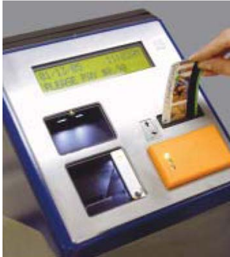
Figure 19 - SL4/5 buses' multi mode-of-payment electronic farebox
