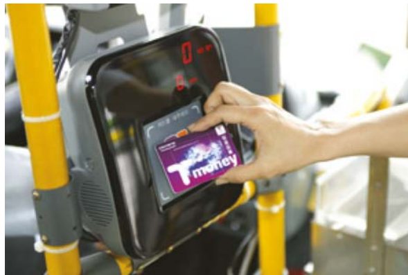
Figure 24 - Electronic farebox for T-Money at Seoul BRT vehicles
