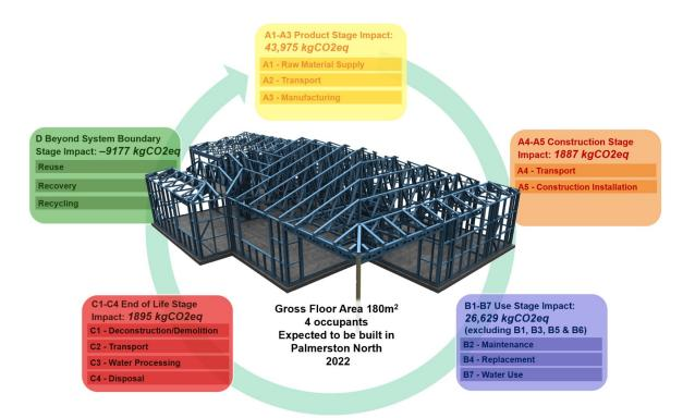
Figure 4. Schematic diagram of absolute climate change potential for each life cycle stage.
