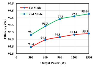
**FIGURE 7.** The efficiency of the diamond shaped MLI under different operating power.
