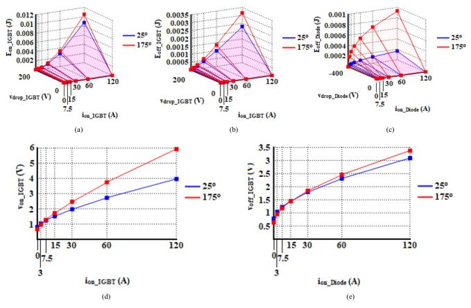
FIGURE 6. Thermal profile of: (a) IGBT turn-on losses, (b) IGBT turn-off losses, (c) diode turn-off losses, (d) IGBT conduction losses and (e) diode conduction losses.
