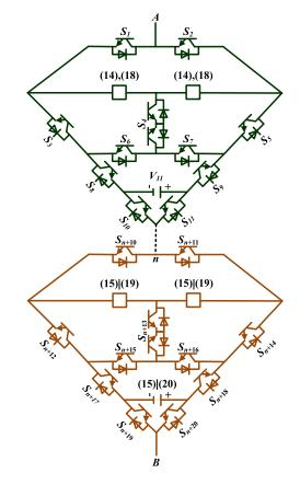
FIGURE 5. The modularity of the proposed diamond shaped MLI.
