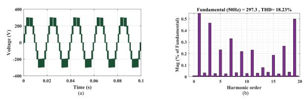
FIGURE 10. Simulation results of diamond-shaped MLI at 1<sup>st</sup> mode: (a) 7-level output voltage, (b) harmonic spectrum.
