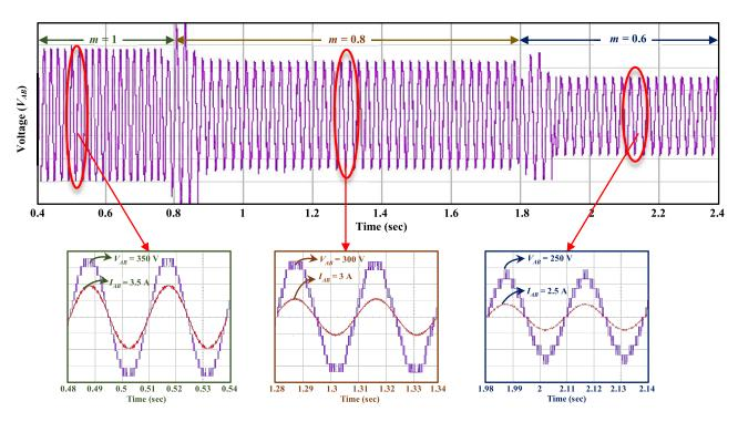
FIGURE 16. Transient performance analysis of diamond shaped MLI under variable modulation index.
