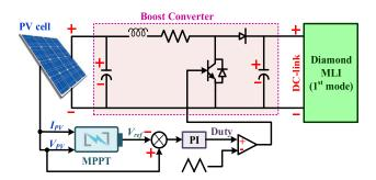
FIGURE 12. PV integration with the diamond shaped MLI.
