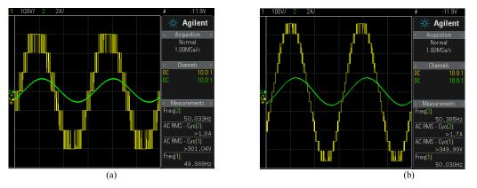
**FIGURE 18.** Experimental results of output voltage (yellow) and current (green) at pf = 0.8: (a) 1<sup>st</sup> mode, (b) 2<sup>nd</sup> mode.
