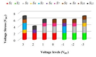
FIGURE 3. Voltage stress under different switches for 1st mode operation.
