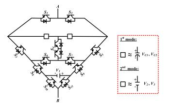
**FIGURE 1.** Schematic diagram of the proposed diamond-shaped multilevel inverter.
