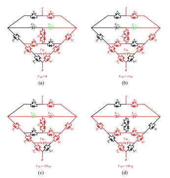
FIGURE 2. Switching operations and current paths of diamond shaped MLI for the positive cycle in 1st mode operation: (a) zero voltage, (b) 1st voltage level, (c) 2nd voltage level, (d) 3rd voltage level.
