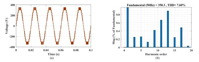
FIGURE 11. Simulation results of diamond-shaped MLI at 2<sup>nd</sup> mode: (a) 15-level output voltage, (b) harmonic spectrum.
