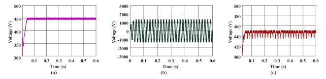
FIGURE 14. Simulation results of PV integrated diamond MLI: (a) DC-link voltage, (b) output voltage, (c) capacitor voltage.
