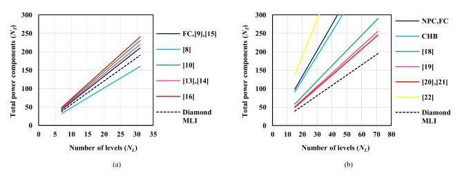
FIGURE 8. Comparison between MLIs in terms of total power components: (a) 1st mode, (b) 2nd mode.
