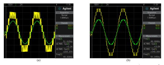
**FIGURE 17.** Experimental results of output voltage (yellow) and current (green) at  $f_{SW} = 5$  kHz: (a) 1<sup>st</sup> mode, (b) 2<sup>nd</sup> mode.
