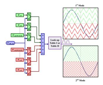
FIGURE 9. The control diagram of SPWM and carrier wave generation.
