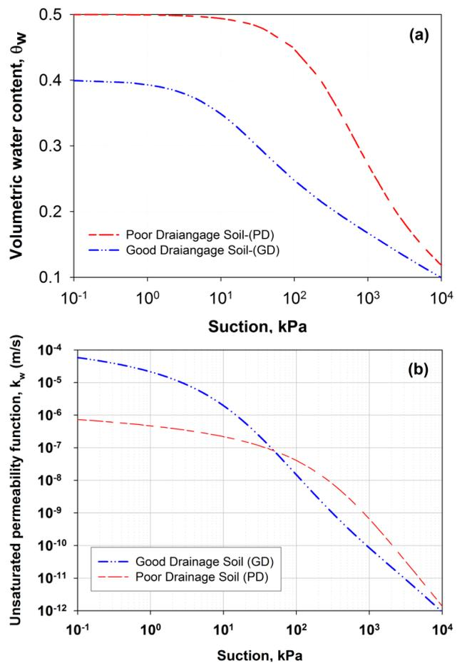
Figure 2. Soil hydraulic properties of GD and PD soils used in numerical modelling: (a) soil-water characteristic curve, (b) unsaturated permeability function
