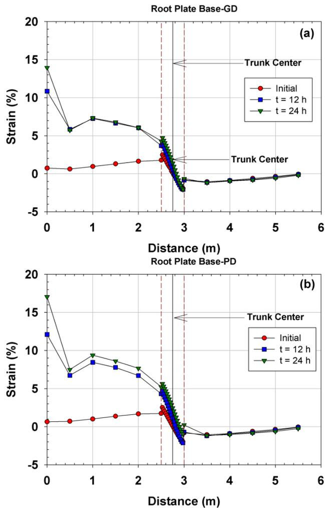
Figure 6. Strains profile in the root plate base: (a) GD soil, (b) PD soil
