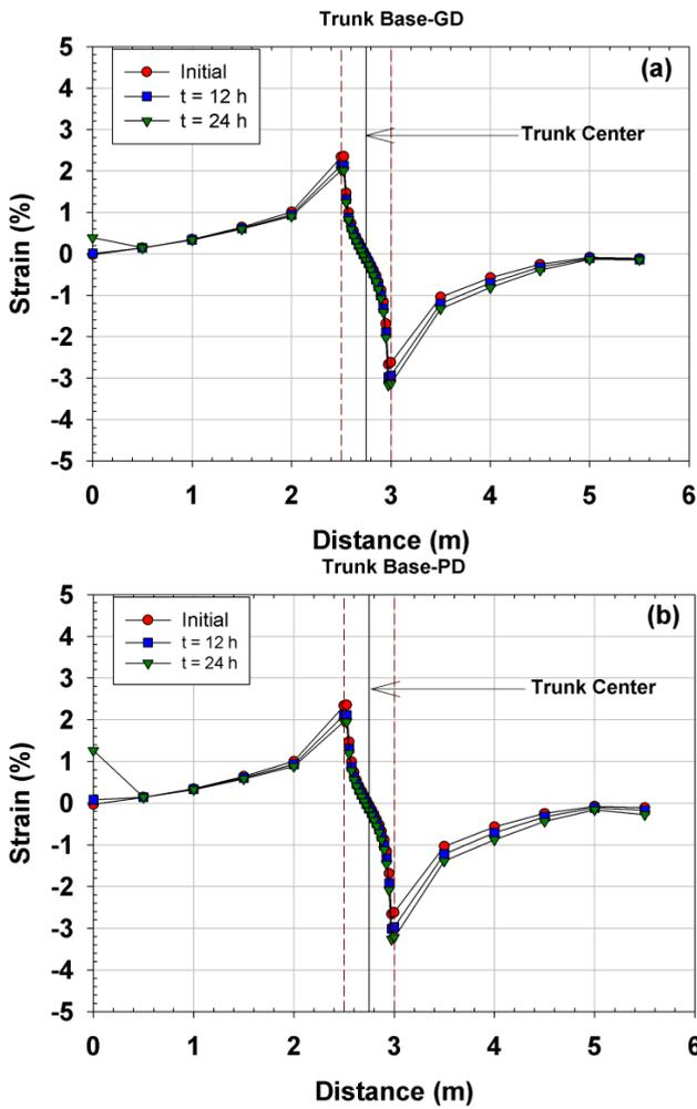
Figure 5. Strains profile in the trunk base: (a) GD soil, (b) PD soil.
