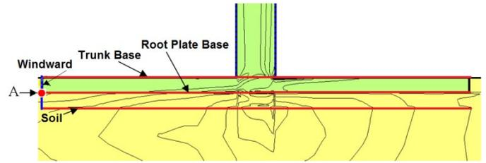
Figure 4. Location of the observed strains in the trunk base, root plate base and soil
