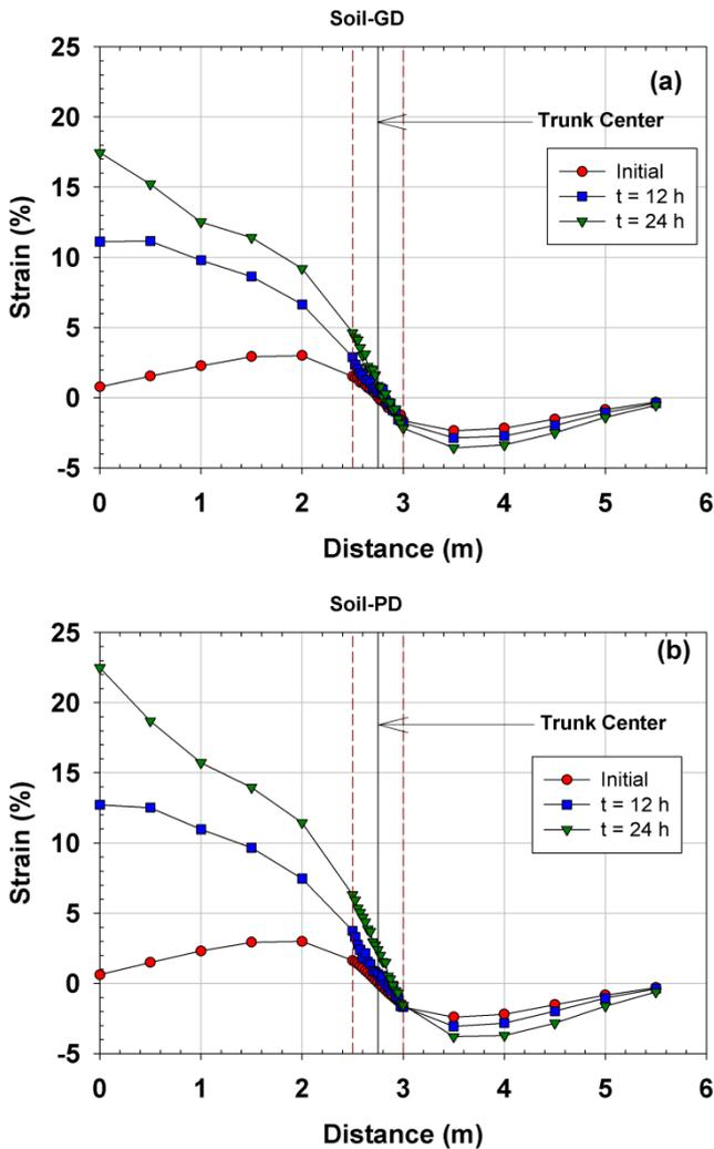
Figure 7. Strains profile in the soil: (a) GD soil, (b) PD soil
