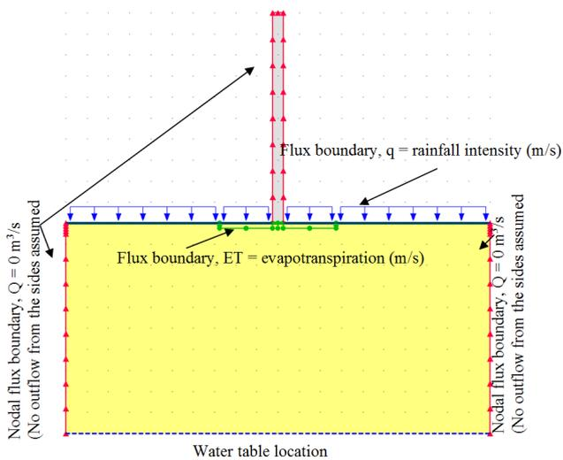
Figure 1. Finite element model and initial condition for the tree-root-soil model
