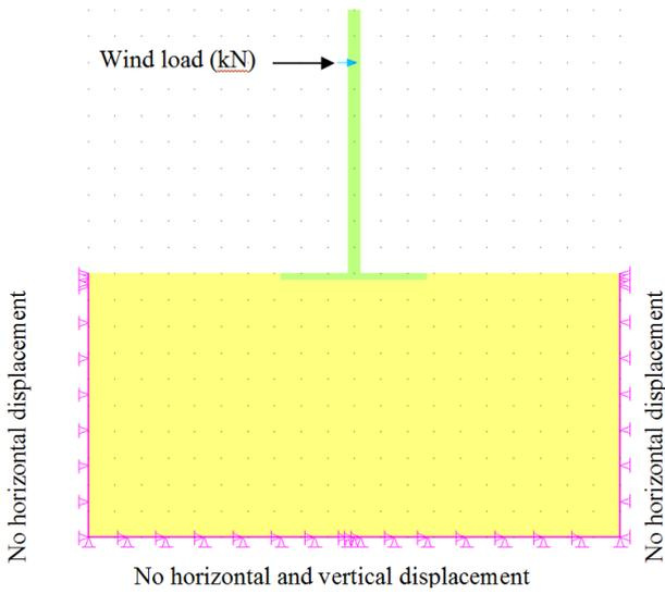
Figure 3-Boundary condition and schematic diagram of tree-root-soil model used in load/deformation analyses
