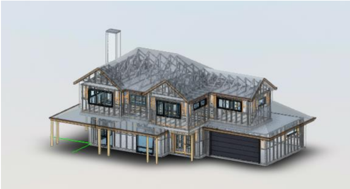
Figure 9 Two-story residential house BIM model
