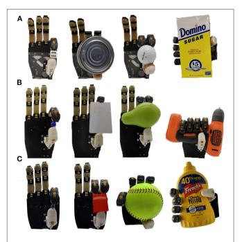
FIGURE 12 | Grasping experiments conducted with the three prosthetic hands equipped with the proposed differential mechanisms whiffletree (A), four output gear differential (B), and series elastic (C). The three differentials can be seen allowing a prosthetic hand to execute a variety of grasping strategies (pinch, tripod, and power grasps).
