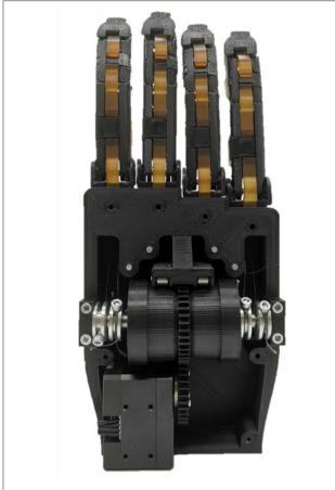
**FIGURE 2** The four-output gear differential can be integrated into a prosthetic hand with the four outputs connected to the index, middle, ring, and pinky fingers. A single motor is used to distribute the load of the actuator to the four fingers through the outer gear module of the differential case.
