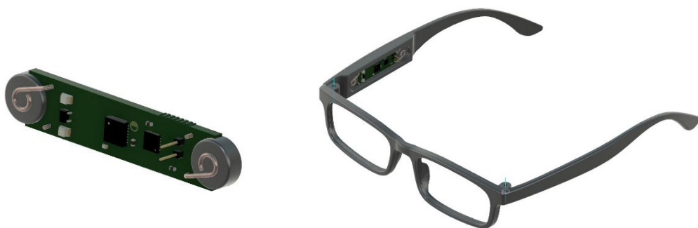
17A. Electronics board for a capacitive sensor 17B. Side arm housing for the electronics board
