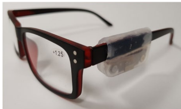
Figure 13. SpecsOn monitor attached to the side arm of the spectacle frame.
