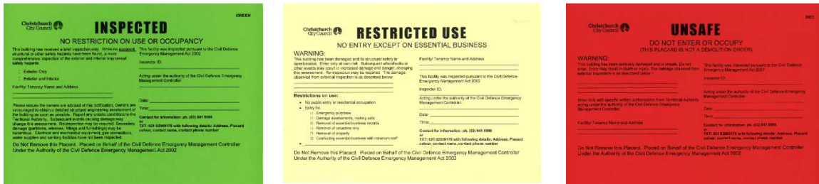
Figure 2. Building assessment notices.
