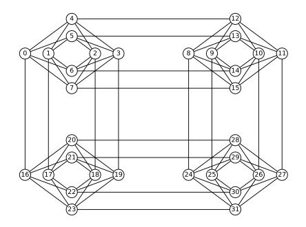
Figure 1: Chimera graph  $\chi_2$  consisting of four  $K_{4,4}$  blocks. In general, the graph  $\chi_k$  consists of a  $k \times k$  grid of such blocks, with connections between adjacent blocks as shown.
