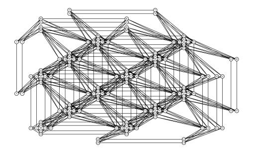
Figure 2: Pegasus graph  $\phi_3$ . In general, the graph  $\phi_k$  is much denser when compared with a Chimera graph with similar order. D-Wave Advantage has a  $\phi_{16}$  chipset.
