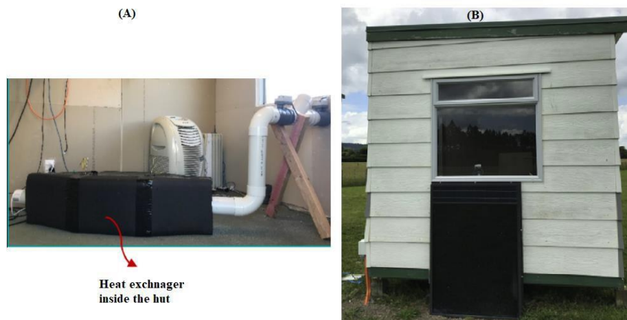
Fig. 4.1. Experimental set up including a PCM heat exchanger (A) inside a hut equipped with a solar collector.
