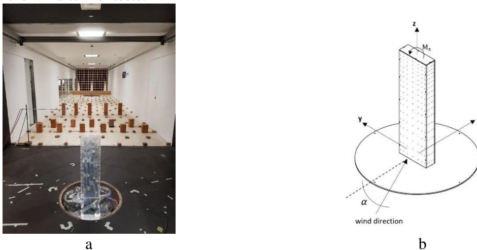
Figure 2. a) Boundary layer wind tunnel setup with HFPI rigid model, b) Global reference system of the tests [14].
