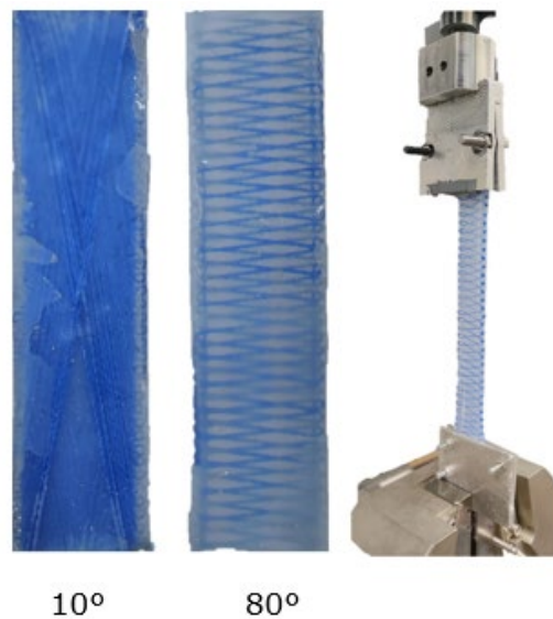
Figure 3.6 Samples of 10^\circ and 80^\circ fibre braided Ecoflex 00-30 with Universal Testing Machine set-up.
