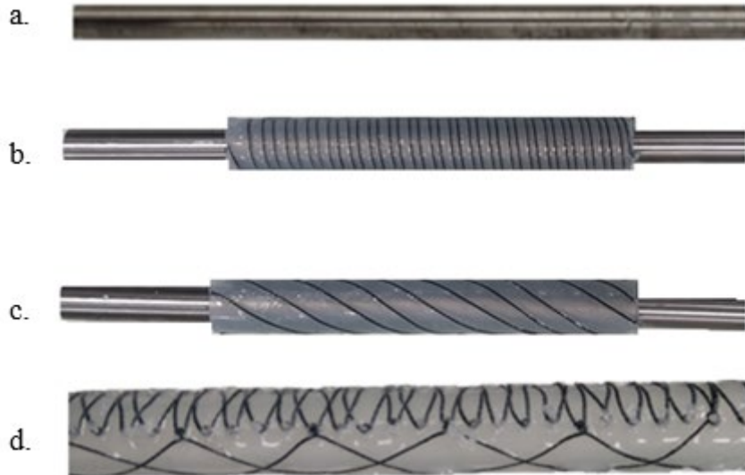
Figure 5.9 Fabrication procedure of SFR actuator. (a) Steel rod (b) Fibres wound at 70°(c) Fibres wound at 10° (d) SFR actuator after winding.
