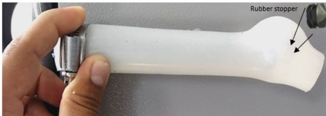
Figure 5.15 Stress at the tip of the actuator resulting in bulging.
