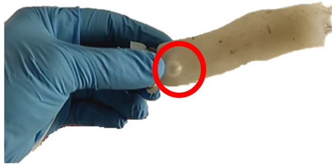
Figure 5.14 Bubbles leading to actuator failure.
