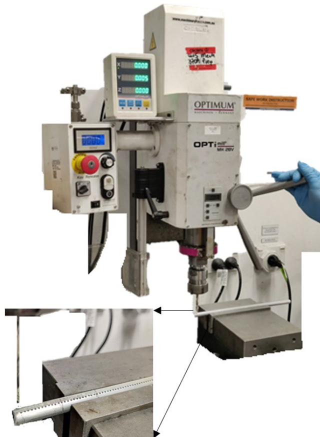
Figure 5.19 Drilling 1mm holes on the aluminium rod using a mill.
