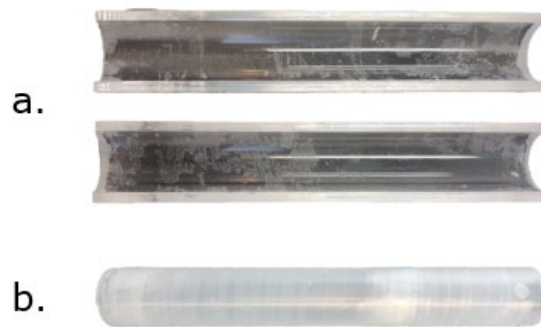
Figure 5.3 Acrylic mould (a) acrylic mould cut along the axis into two halves (b) taped around to bind the two halves together.
