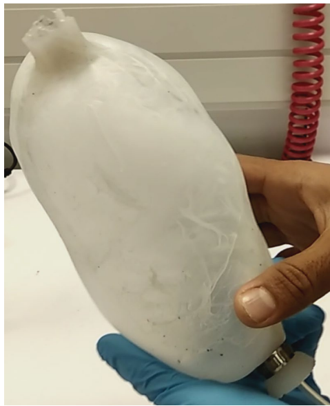
Figure 5.18 Bulging in SFR actuator at pressure above 80 kPa.
