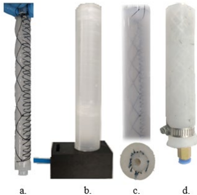
Figure 5.10 Demonstrates the coating of the final layer of Ecoflex™ 00-30 to finish SFR actuator. (a) SFR actuator before the final layer of Ecoflex™ 00-30 (b) 30 mm mould (c) Cross-sectional view of the actuator (d) SFR actuator after final layer of Ecoflex™ 00-30.
