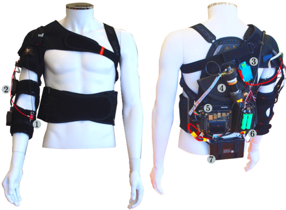
Figure 2.12 Untethered elbow Exo-suit .1. Load cell 2. IMU sensors 3. Load cell amplifier 4. Actuation stage 5. Embedded controller and motor drive stage 6. Controller battery pack 7. Motor drive battery pack [135].
