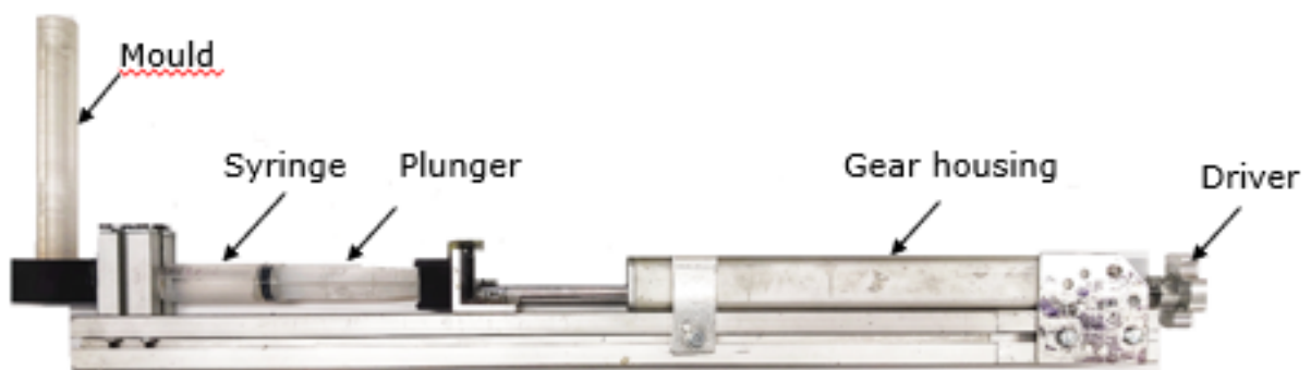
Figure 6.3 Injection moulding device to create a bubble-free actuator.
