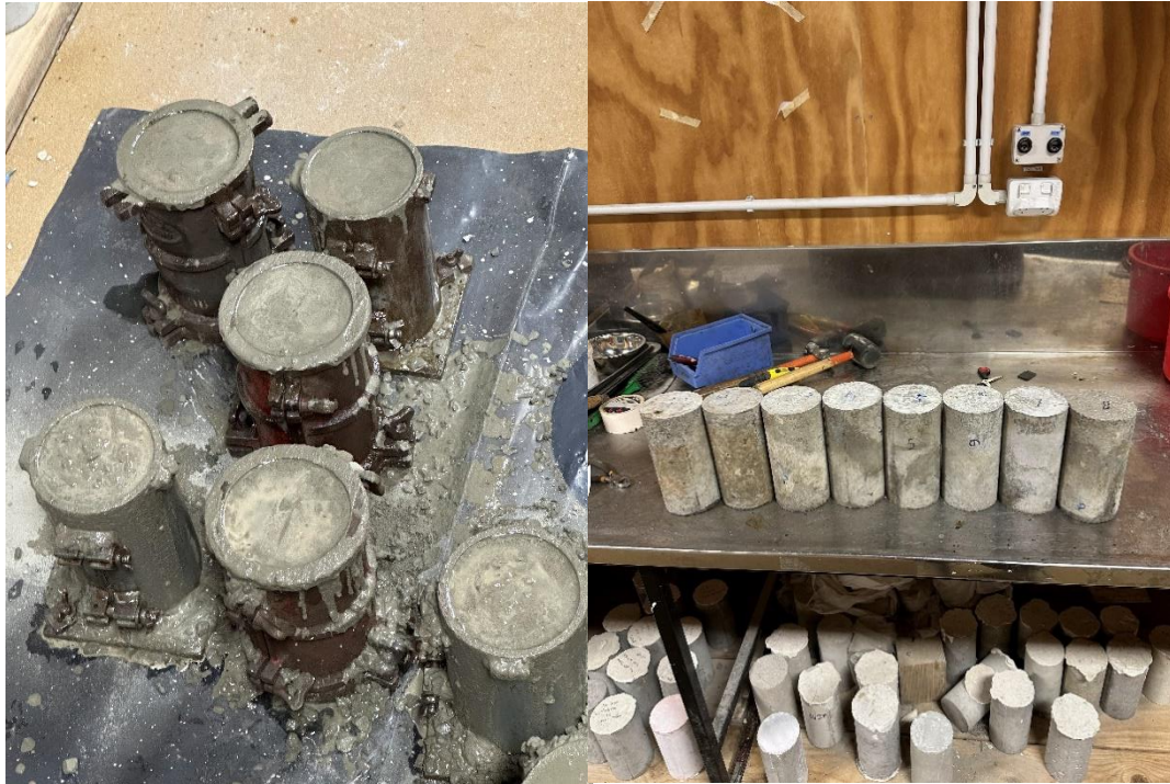
Figure 3-2: Mould Preparing Procedure
