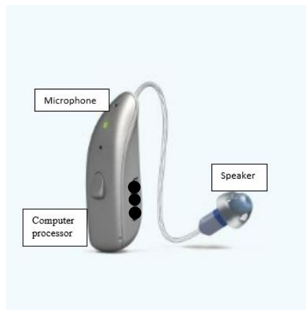
Figure 5: Hearing aid main components
