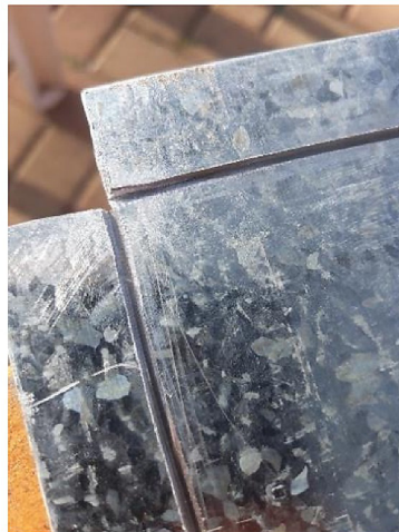
Fig. 2. (a) New base folded and (b) Score lines before folding.
