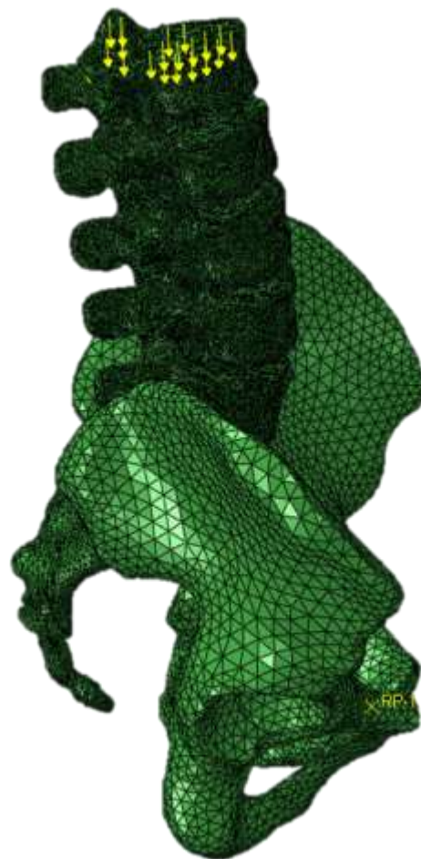
Figure 27: Loading and Boundary conditions applied in the whole lumbar FE model
