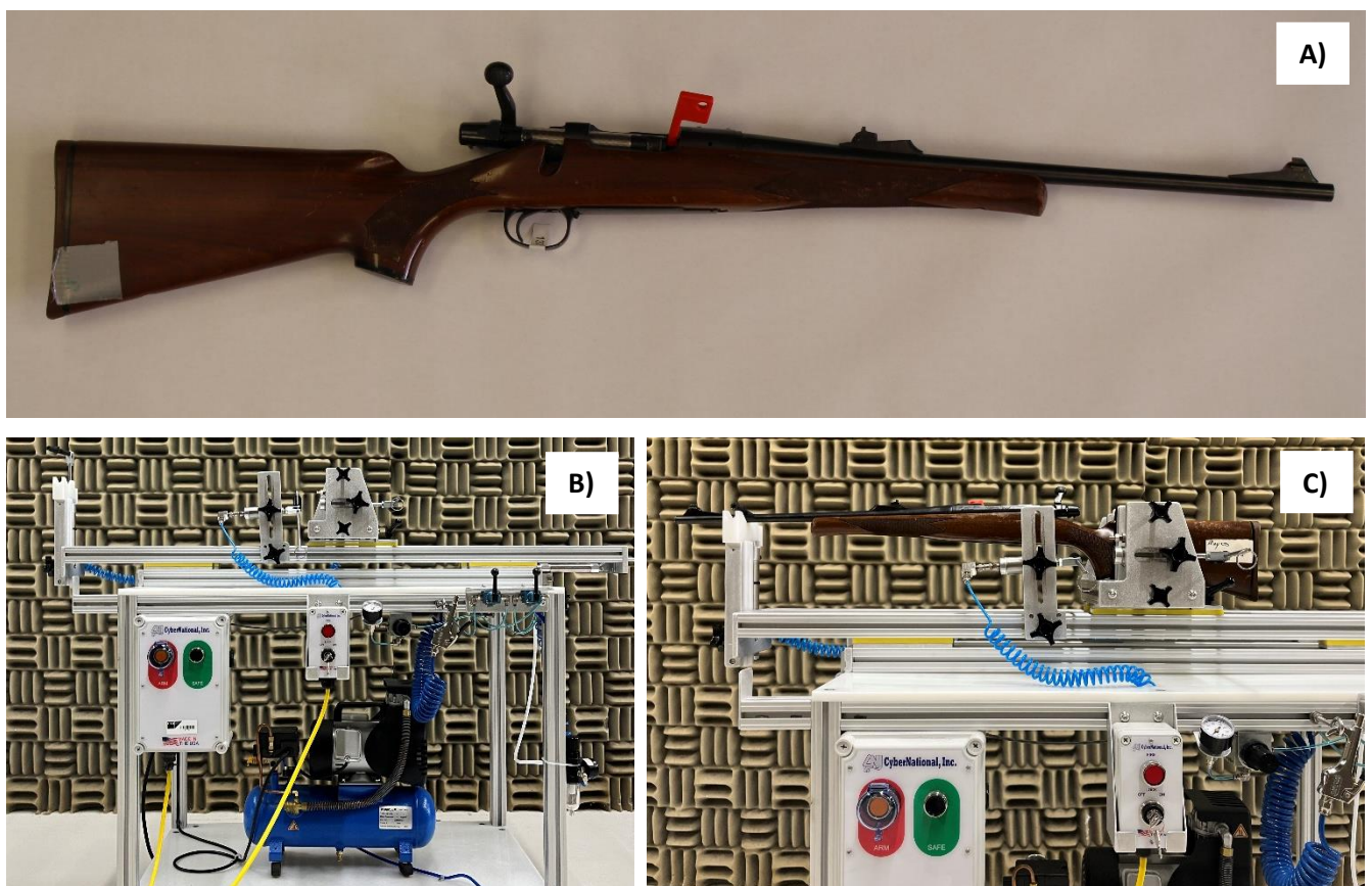
Figure 2.3 Photographs of the firearm and remote firing cart used in this research. A) Remington Model Seven bolt-action .223 Rem calibre rifle B) The remote firing cart used to fire the bolt-action rifle. C) The bolt-action rifle contained within the remote firing cart.
