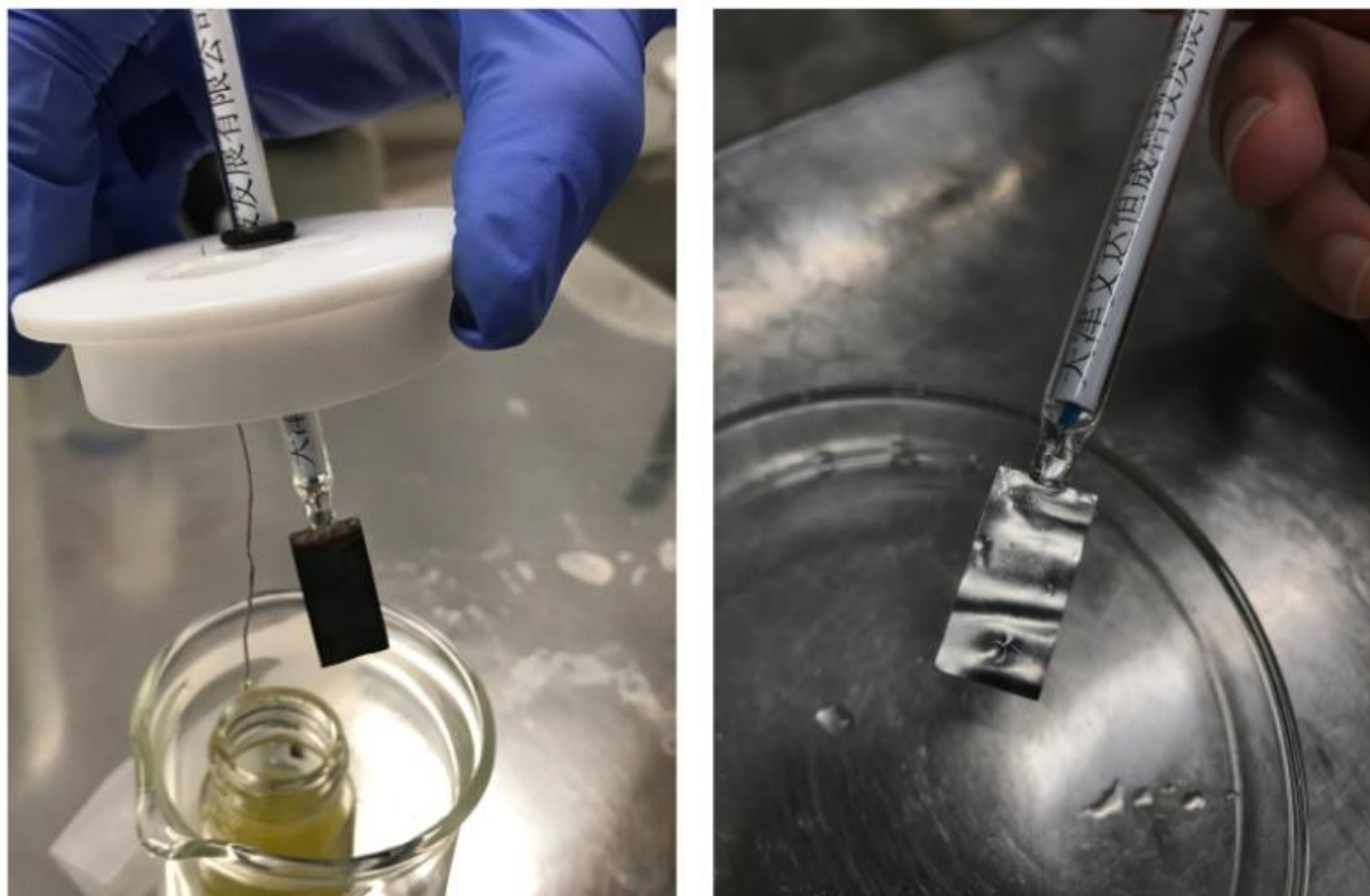
Figure 26. Comparison of platinum plate before and after washing.
