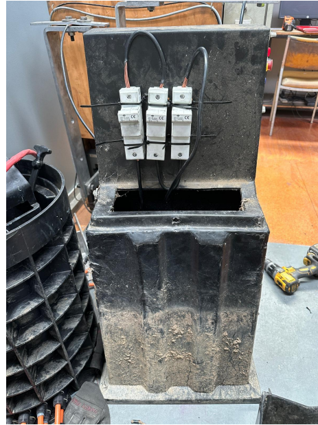
Figure 22 Assembly Single Fuse Holder & Figure 23 Assembly Three Fuse Holders
