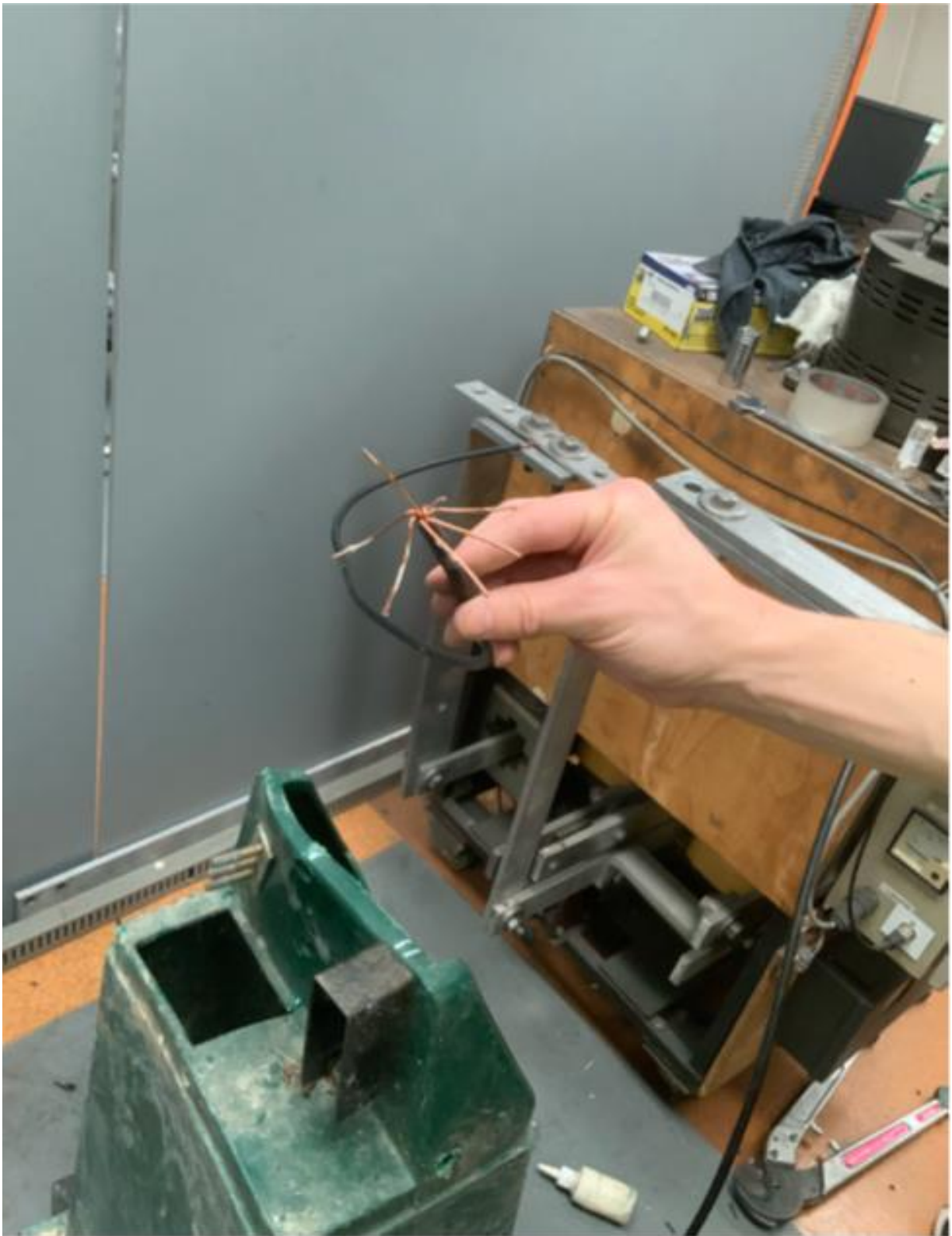
Figure 4 Strand Separation of Copper Cable
