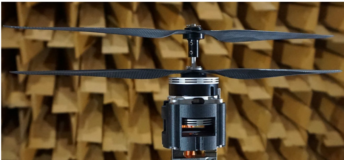
Fig. 1 Photograph of the first contra-rotating UAV rotor system mounted in the anechoic chamber.
