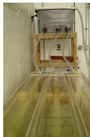
Figure 2.2: High capacity flow chamber, showing channels and header tank.
