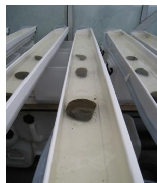
Figure 2.6: Low capacity flow chambers, second setup containing natural substrates.
