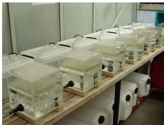
Figure 2.4: Low capacity flow chambers, first setup, in operation.
