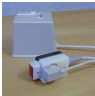
Figure 3.12: Hewlett-Packard S4 Ultrasound transducer with magnetic receiver. The ultrasound transducer (red) with holder (black and white) and the attached Flock of Birds magnetic receiver. The larger square box in the background is the magnetic transmitter.
