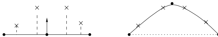
Figure 3.1: Adjusting the nodal parameters of the mesh to minimise the least-squares distance between each data point ( \times ) and its orthogonal projection on the surface. Shown is the effect of adjusting the nodal and derivative parameters of the middle node and the derivative values of the end nodes.
